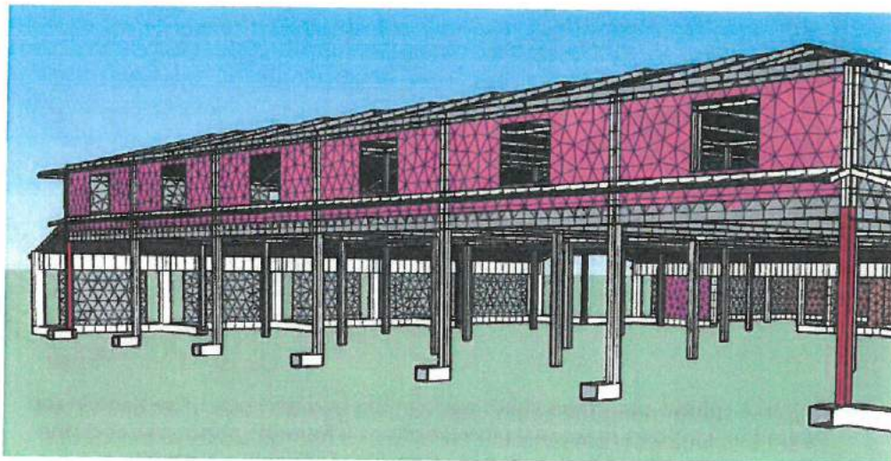
Figure 5. Modeling of second floor perimeter walls (pink) over beams and columns below. Corner columns are shown in red.
